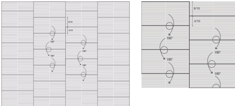
For this size of wall tile, install with the **Litefix** or **Flex GT-30** adhesive mortar. Use a 1/4"x3/8" or 1/2"x1/2" trowel. With the flat side of the trowel, apply, with pressure, a thin layer of mortar and then apply another layer with the notched side of the trowel. Always back-butter the tile with the flat side of the trowel to ensure a strong adhesion.
